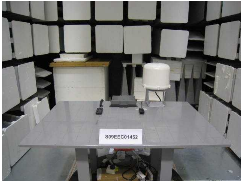
Radiated Emissions Test Setup (Front View)
