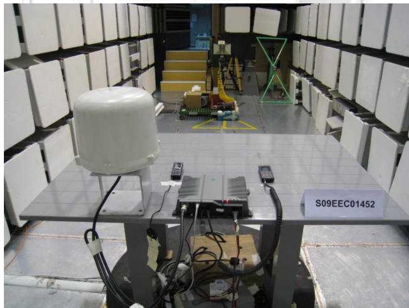
Radiated Spurious Emissions Test Setup (Rear View)
