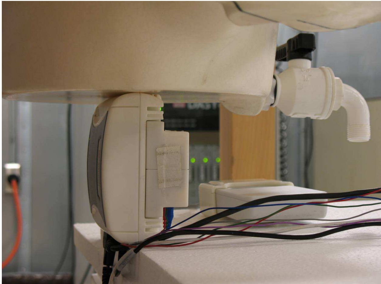
Figure 11: Device Positioning for SAR Scans – Antenna Side Against Phantom
