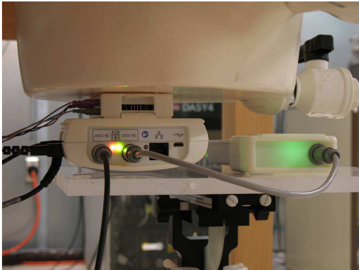
Figure 9: Device Positioning for SAR Scans – Back Side Against Phantom
