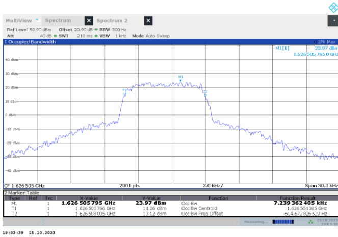
Figure 7.1-19: 99 % bandwidth on low channel for waveform Y
