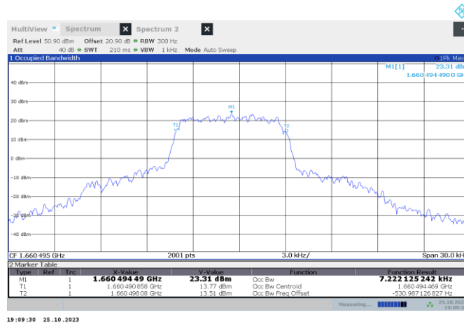
Figure 7.1-21: 99 % bandwidth on high channel for waveform Y
