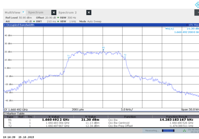
Figure 7.1-27: 99 % bandwidth on high channel for waveform Z
