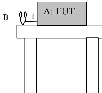
\*The test without Cradle had a worst noise level, so that the test was performed with above setup (without connecting USB cable).
