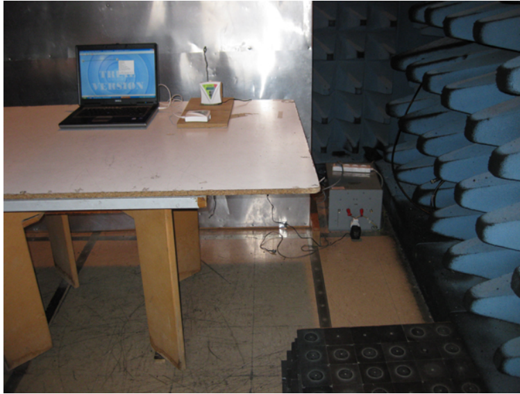
Figure 2. Conducted Emission Tested Setup
