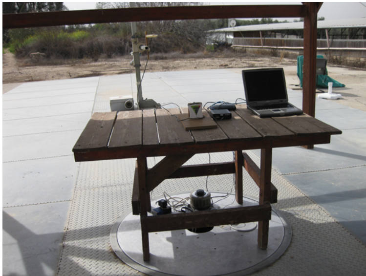
Figure 3. Radiated Emission Test Setup
