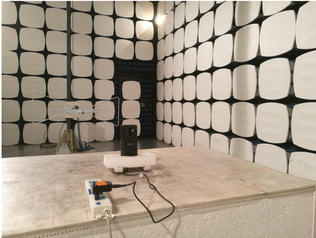
Radiated Spurious Emission Below 1GHz
