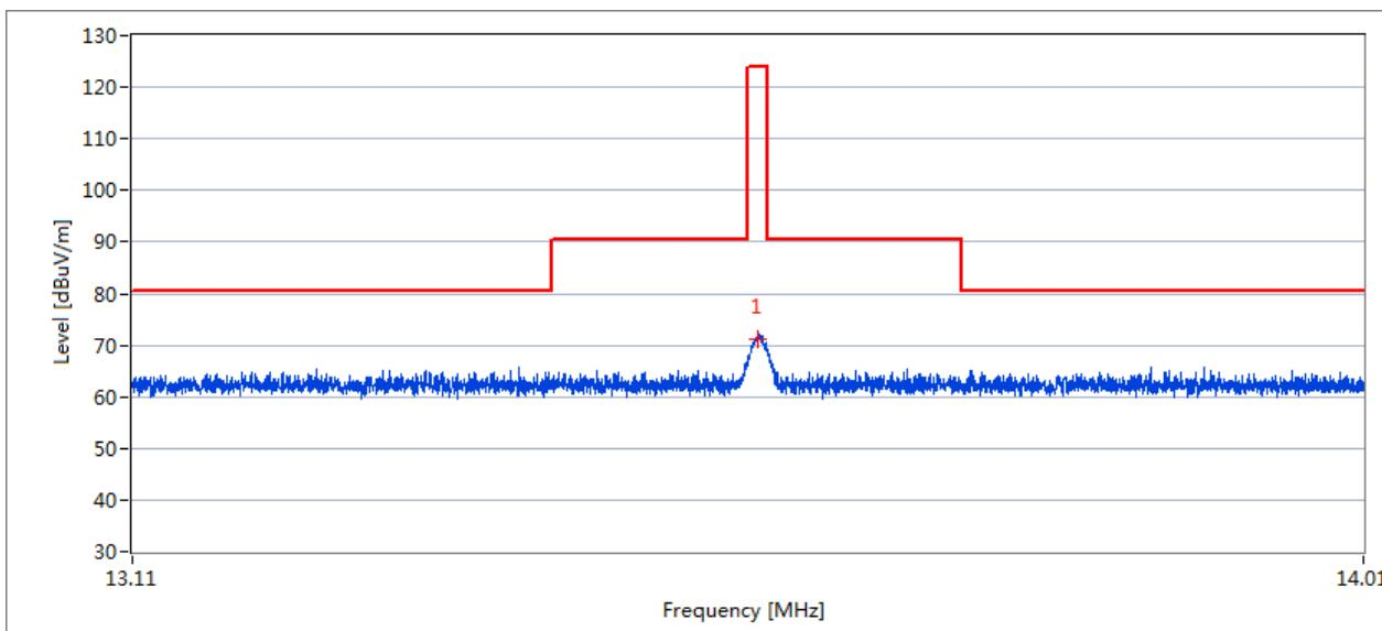
Spurious emissions at 9kHz~13.110MHz & 14.010MHz~30MHz
