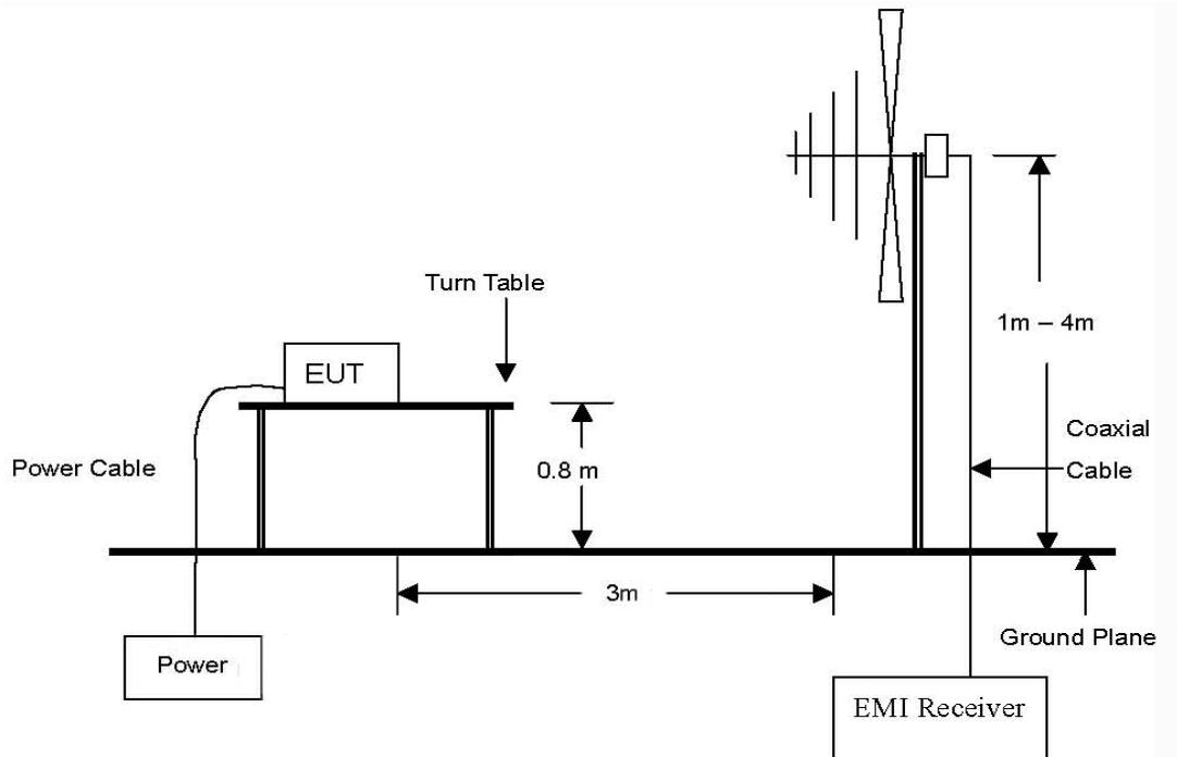
The diagram below shows the test setup that is utilized to make the measurements for emission from 1 GHz to 24 GHz Emissions.
