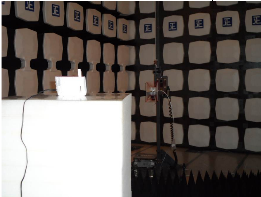
Measurement of Radiated Emission Test Set Up
