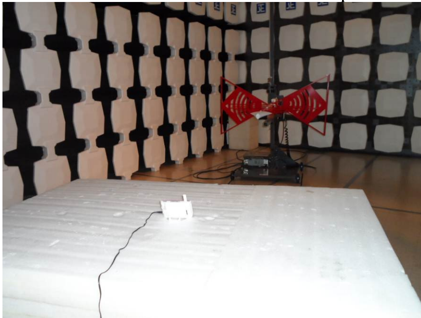
Measurement of Radiated Emission Test Set Up
