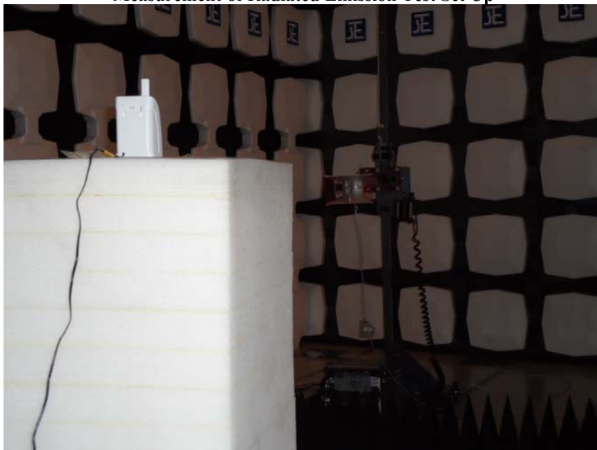
Measurement of Radiated Emission Test Set Up
