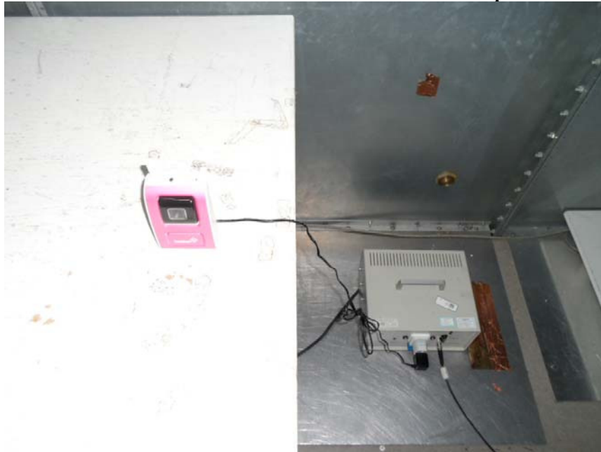
Measurement of Conducted Emission Test Set Up
