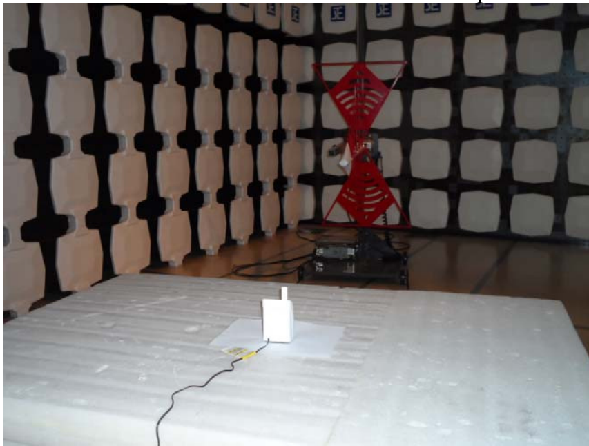
Measurement of Radiated Emission Test Set Up
