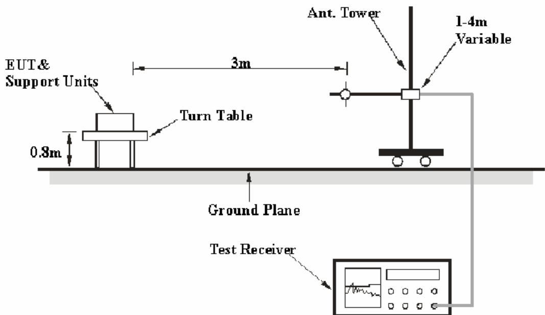
The radiated emission tests were performed in the 3 meters chamber B test site, using the setup accordance with the ANSI C63.4-2003. The specification used was the FCC 15.209, FCC 15.109 and FCC 15.247 limits.
