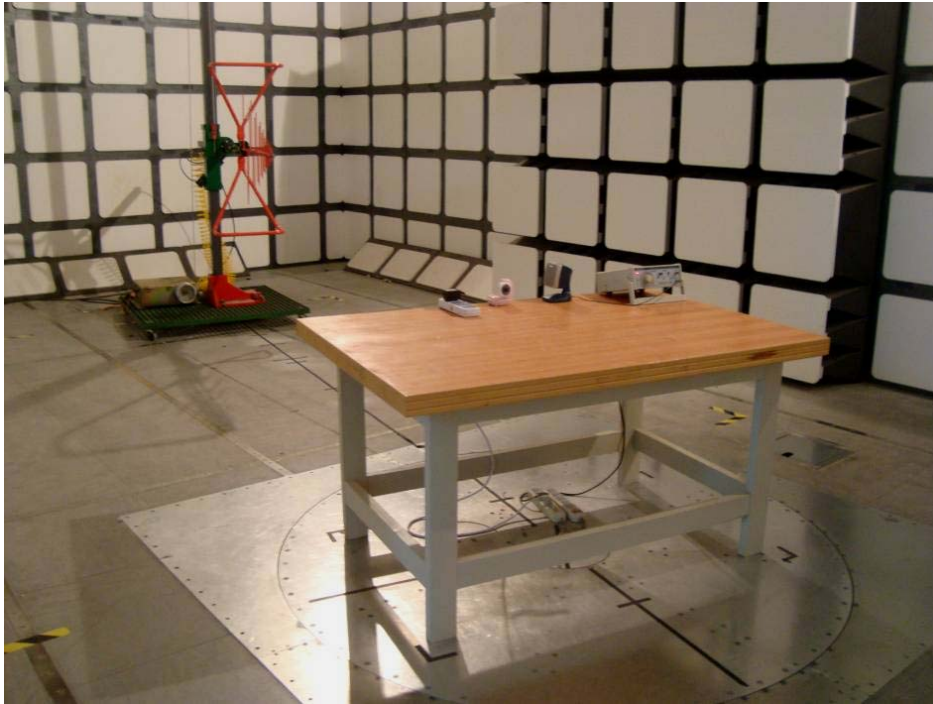
Radiated Emissions – Rear View
