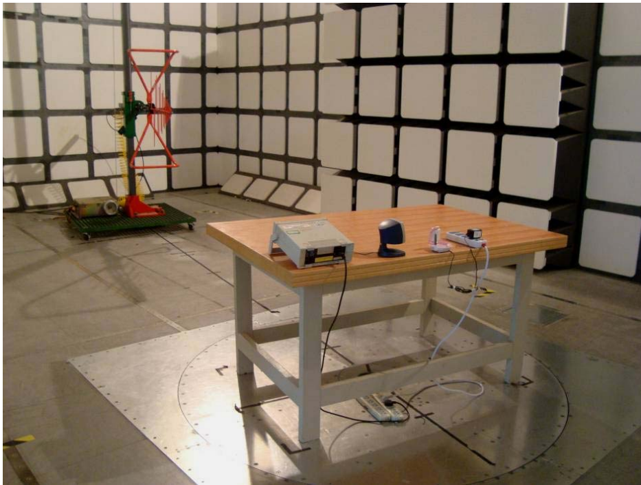
Radiated Emissions – Rear View
