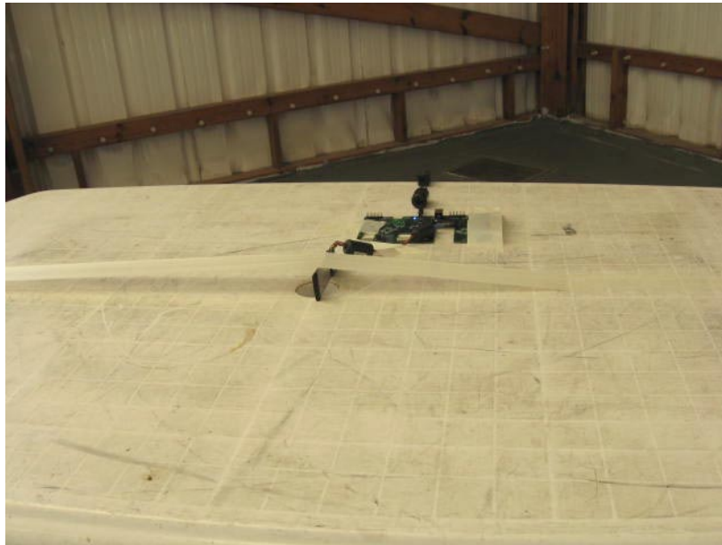
Photograph No.5 Radiated emissions measurement setup at the OATS, EUT close view in Z-axis position
