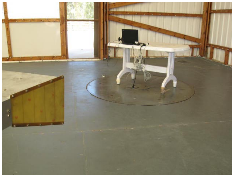
Photograph No.11 Radiated emissions measurement setup at the OATS above 1000 MHz
