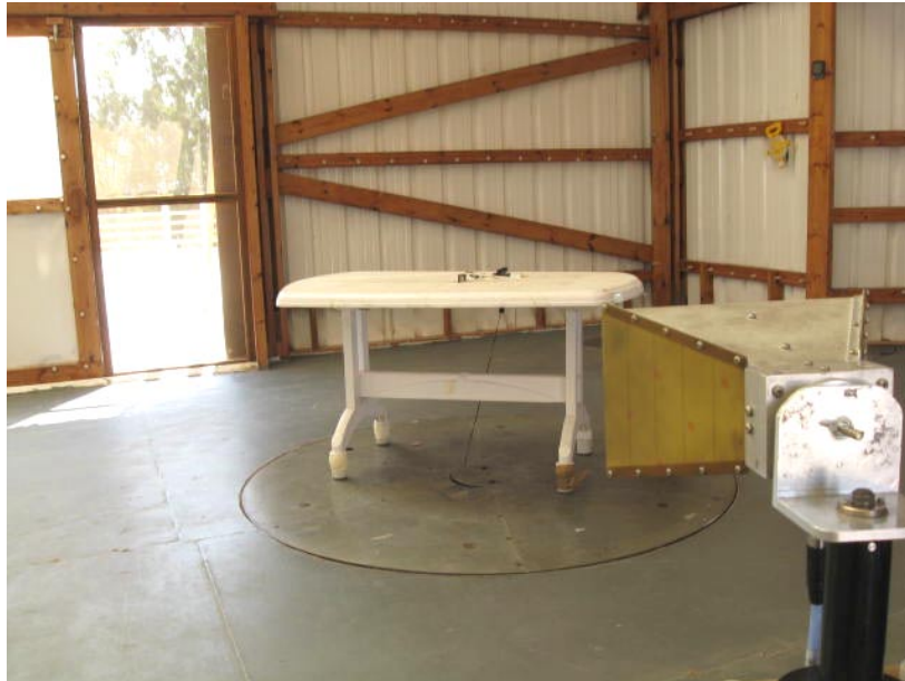
Photograph No.2 Carrier and spurious radiated emissions measurement setup at the OATS
