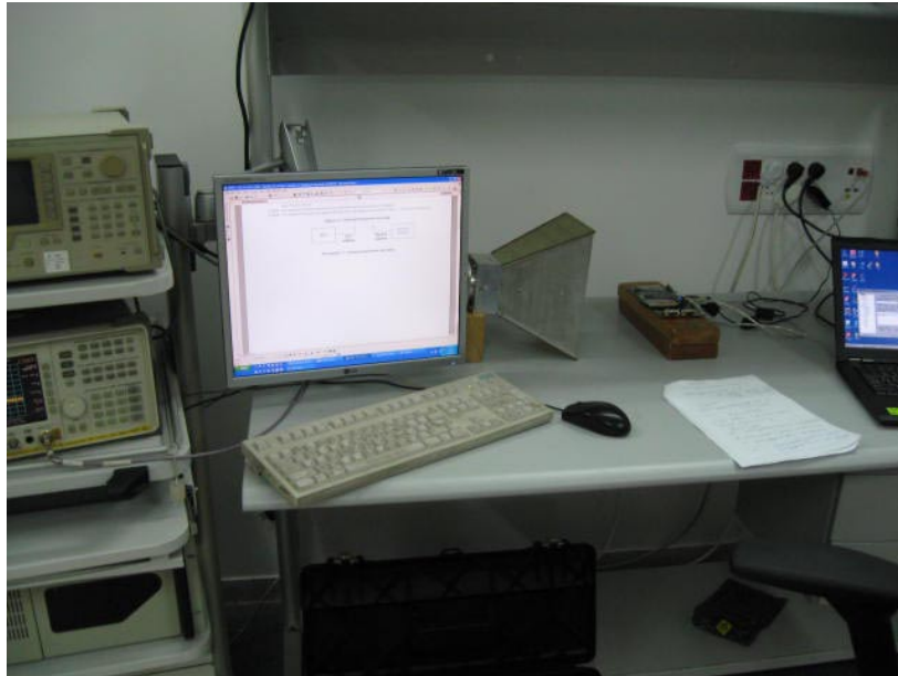
Photograph No.7 Carrier frequency separation, number of hopping frequencies measurement setup
