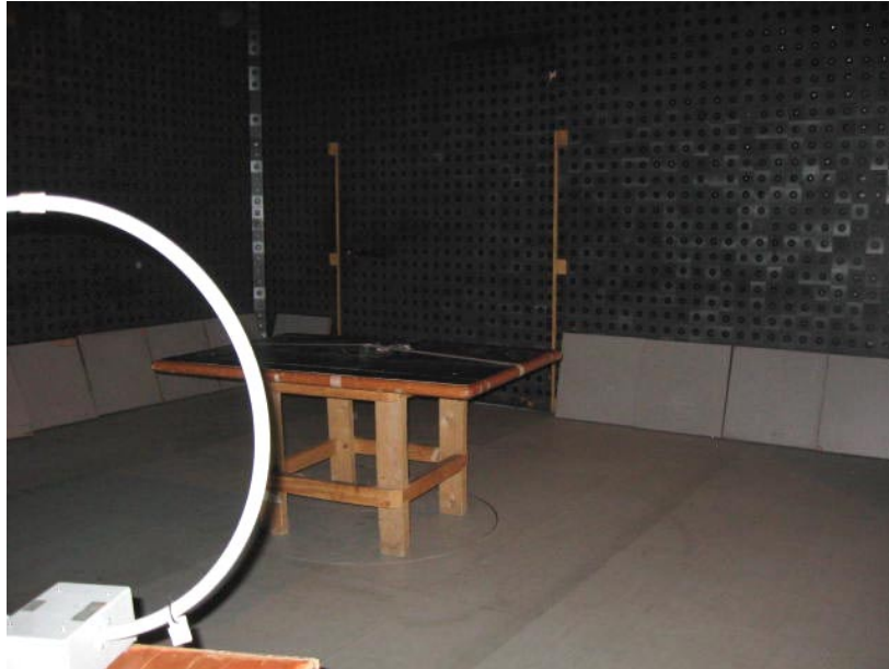
Photograph No.6 Spurious radiated emissions measurement setup in the anechoic chamber below 30 MHz
