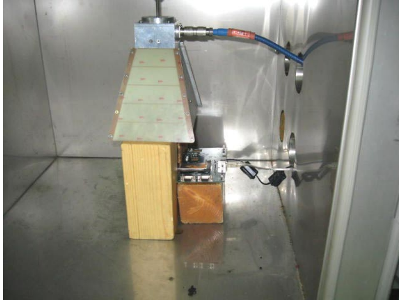
Photograph No.1 Occupied bandwidth measurement setup
