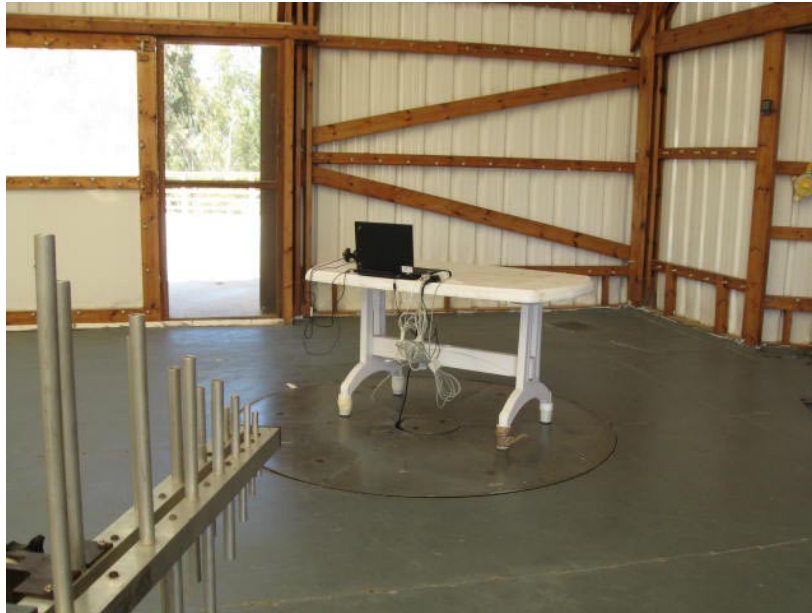
Photograph No.10 Radiated emissions measurement setup at the OATS in 30-1000 MHz
