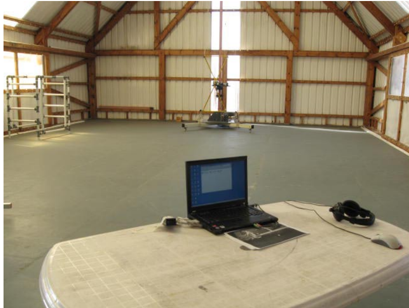
Photograph No.12 Radiated emissions measurement setup at the OATS, EUT close view
