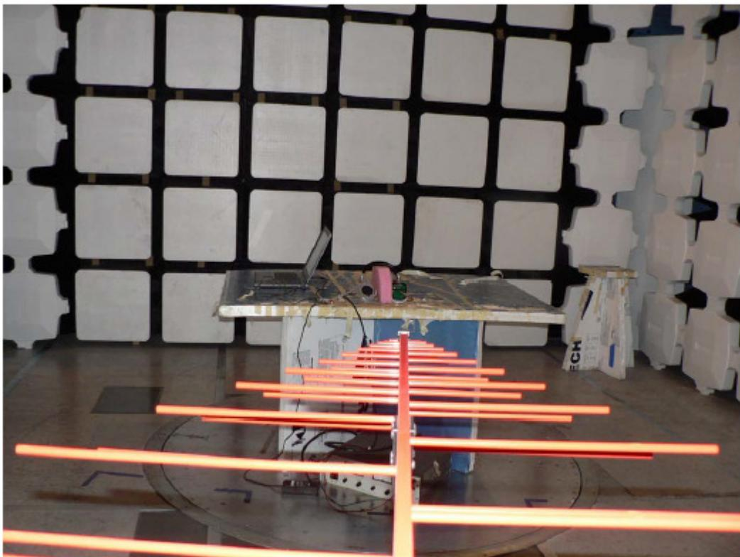
**10.3 Radiated Emissions Test Setup > 1 GHz**
