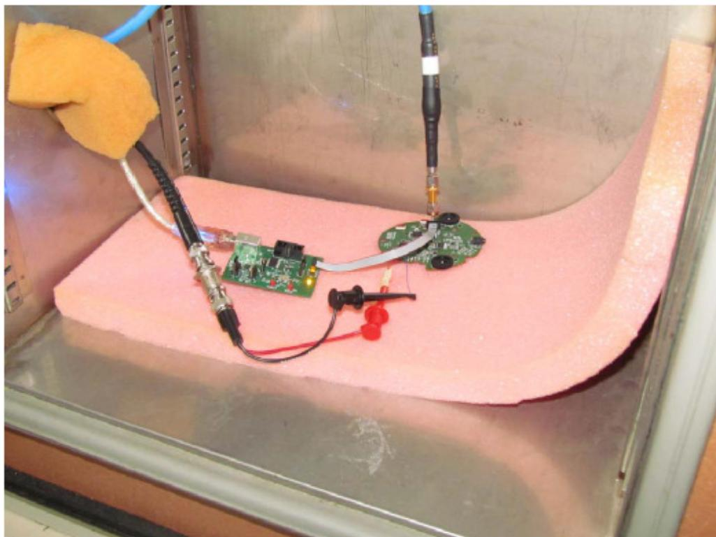
**10.2 Radiated Emissions Test Setup < 1 GHz**
