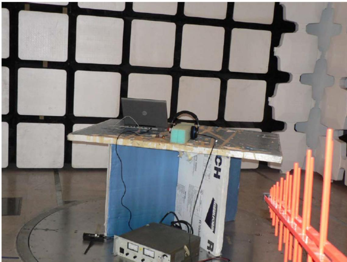
**7.3. Radiated Emissions Test Setup > 1 GHz**
