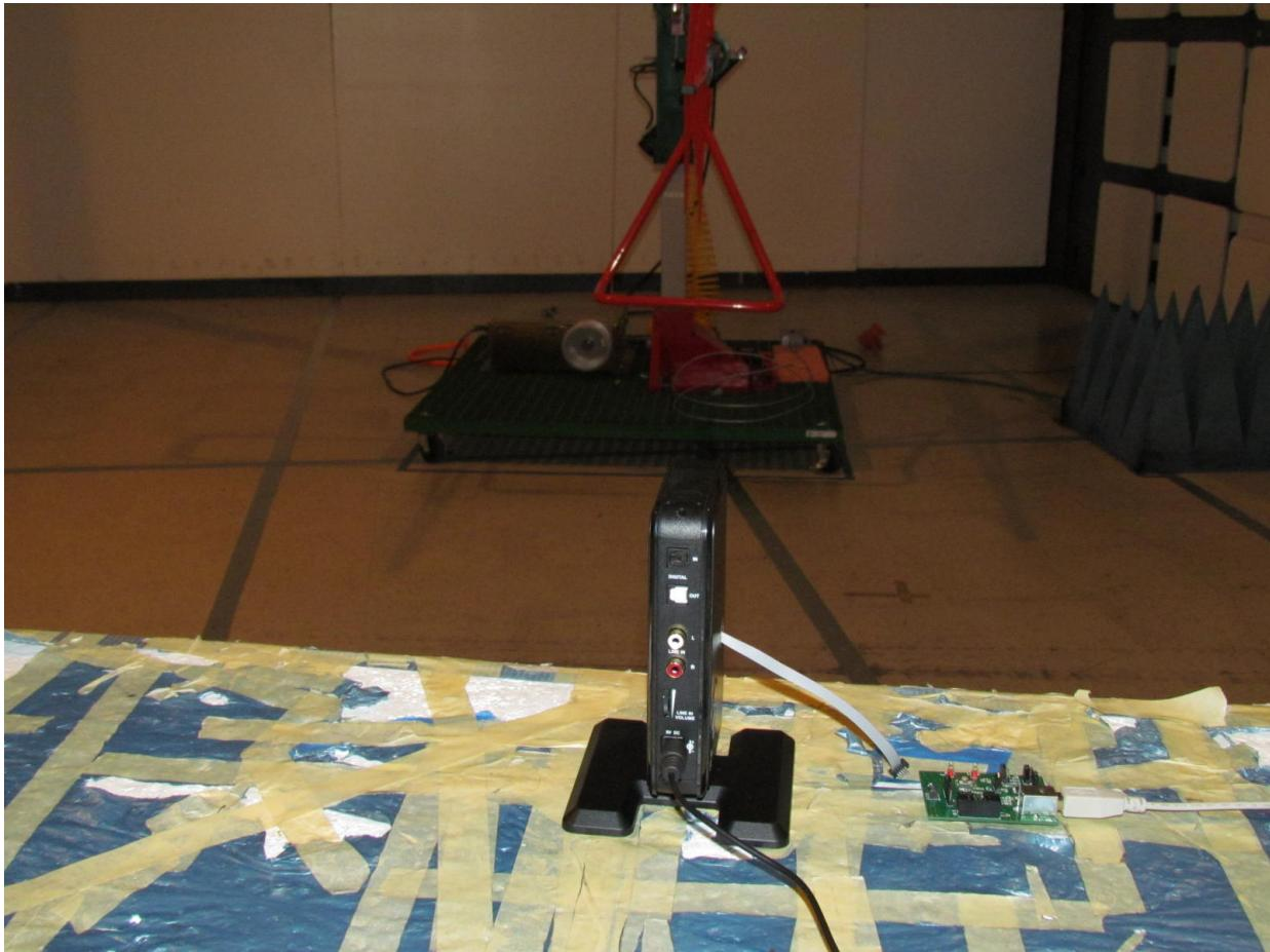
Test Setup - Radiated Emissions > 1 GHz
