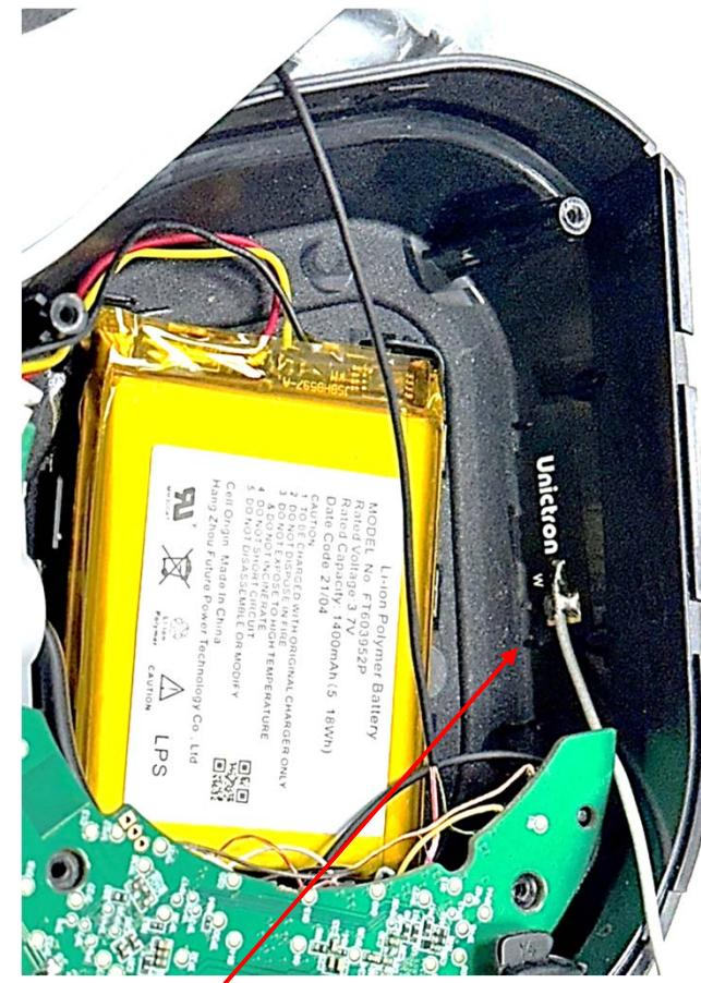
Attach the WW20D0 along the bottom alignment bar and align it with the bottom edge on the side
