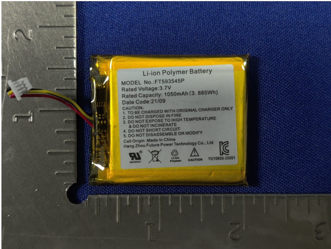
Figure 6: Internal Photo of Stealth700P-MAX-RX – Battery
