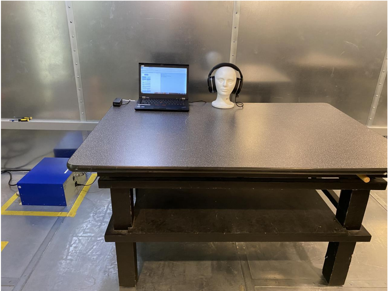
Figure 10: AC Conducted Emission Test Setup (Front View)
