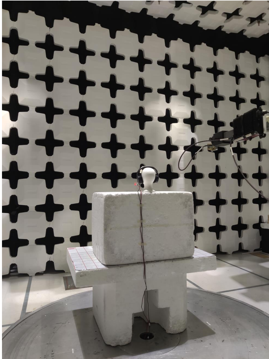
Figure 8: Test Setup for 18 GHz to 26 GHz (Rear View)
