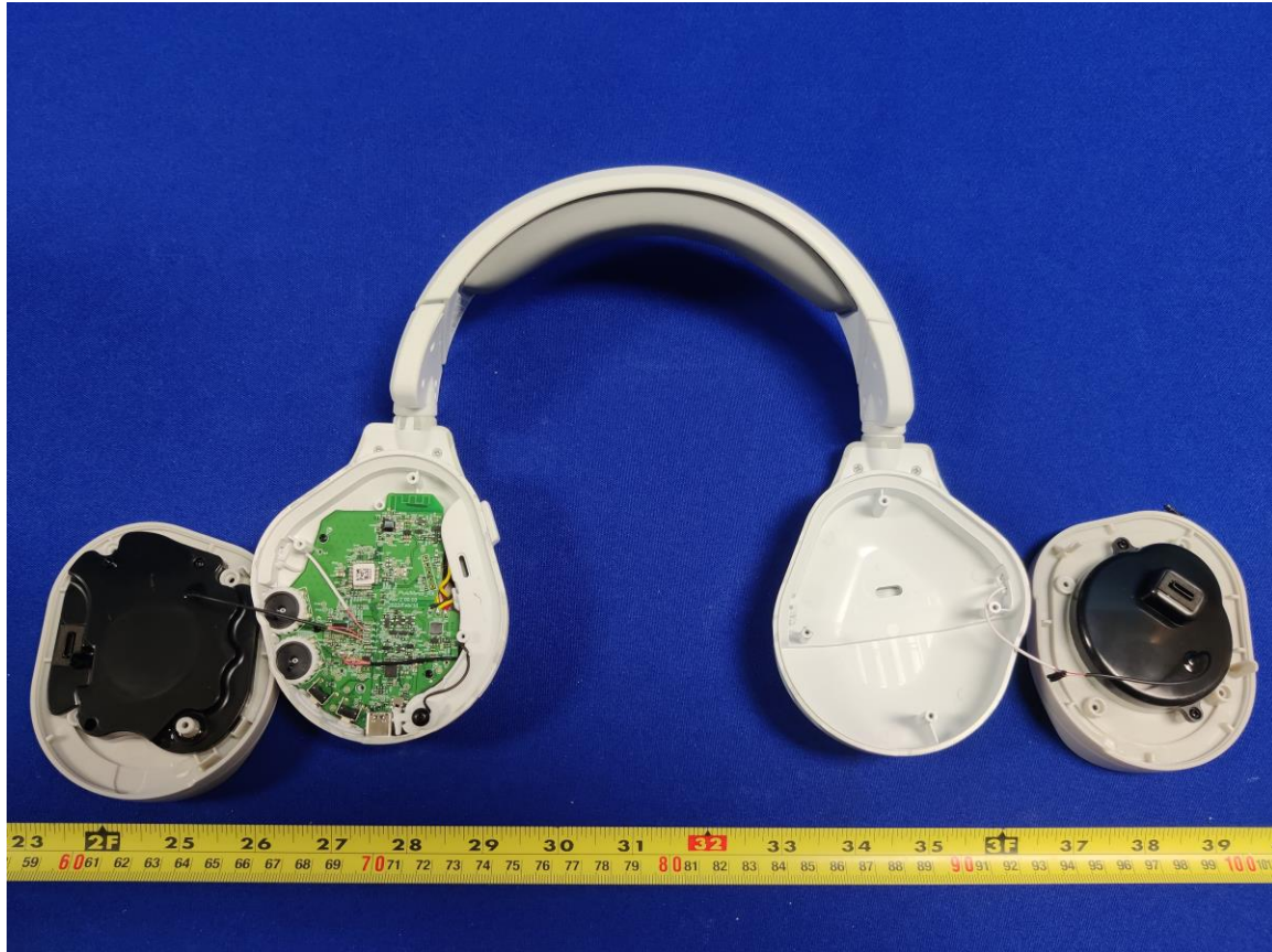
Figure 1: Internal Photo of Stealth600P-MAX-RX with Plastic Cover Removed
