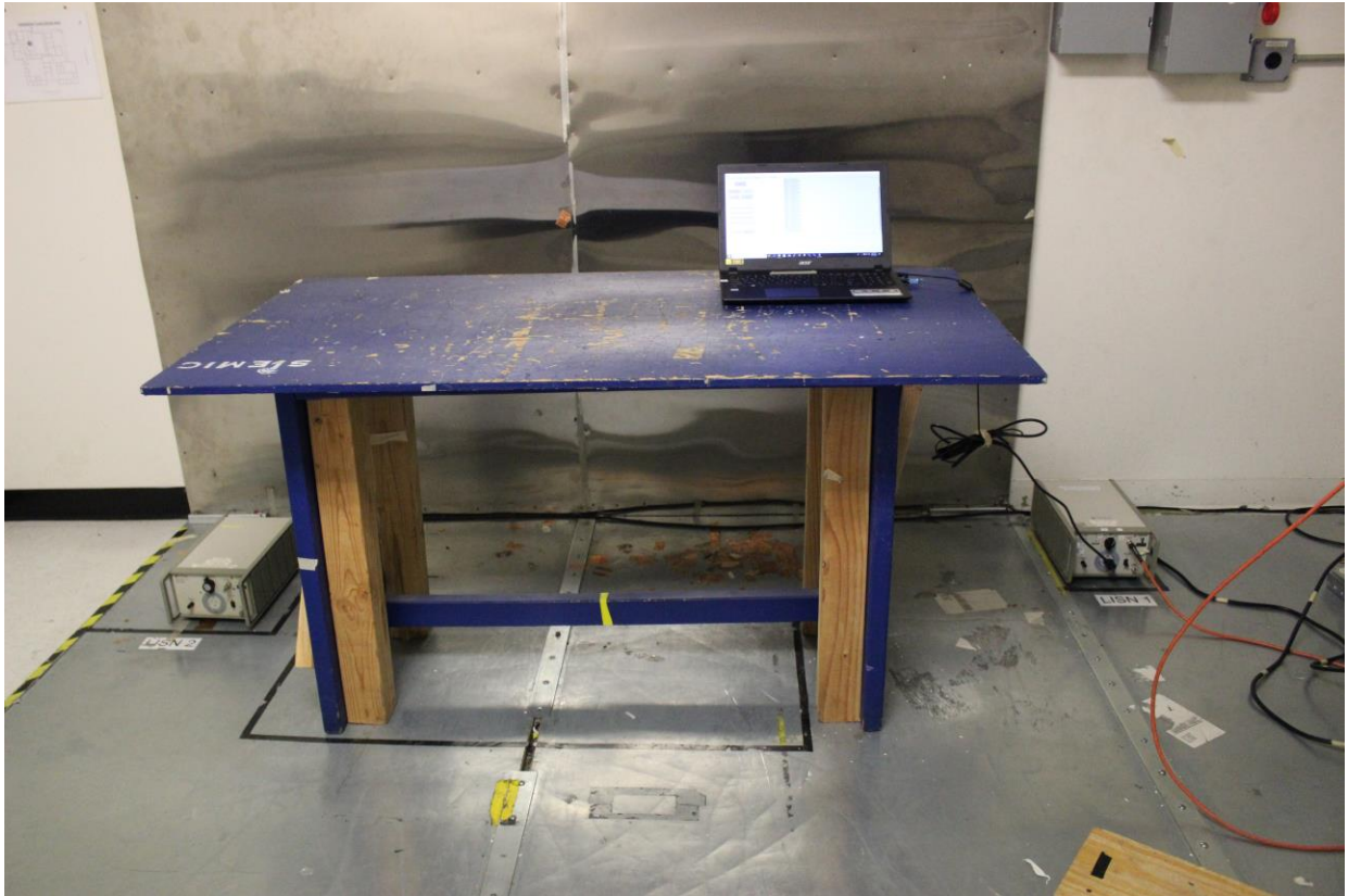
Figure 10: AC Conducted Emission Test Setup (Front)
