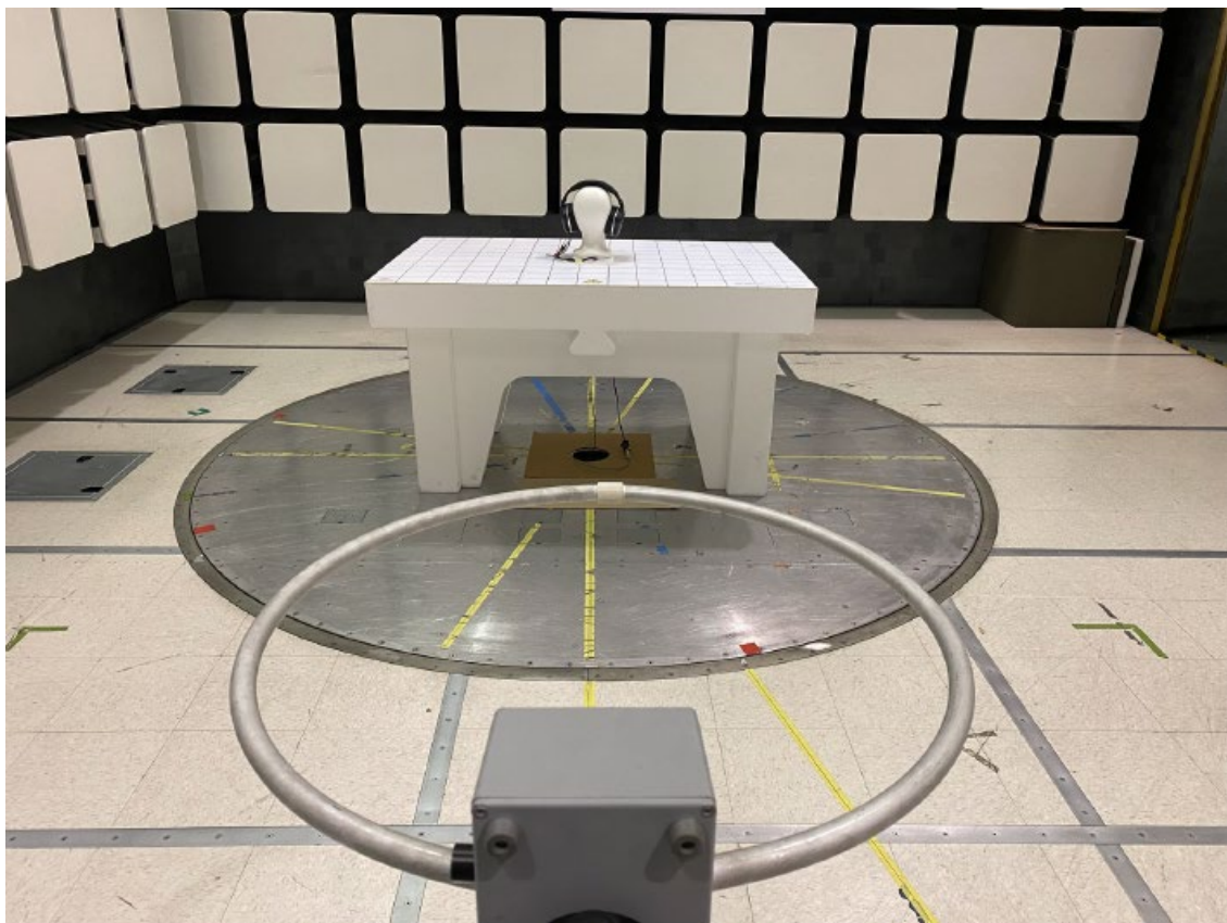
Figure 2: Test Setup for 9 kHz to 30 MHz (Rear View)
