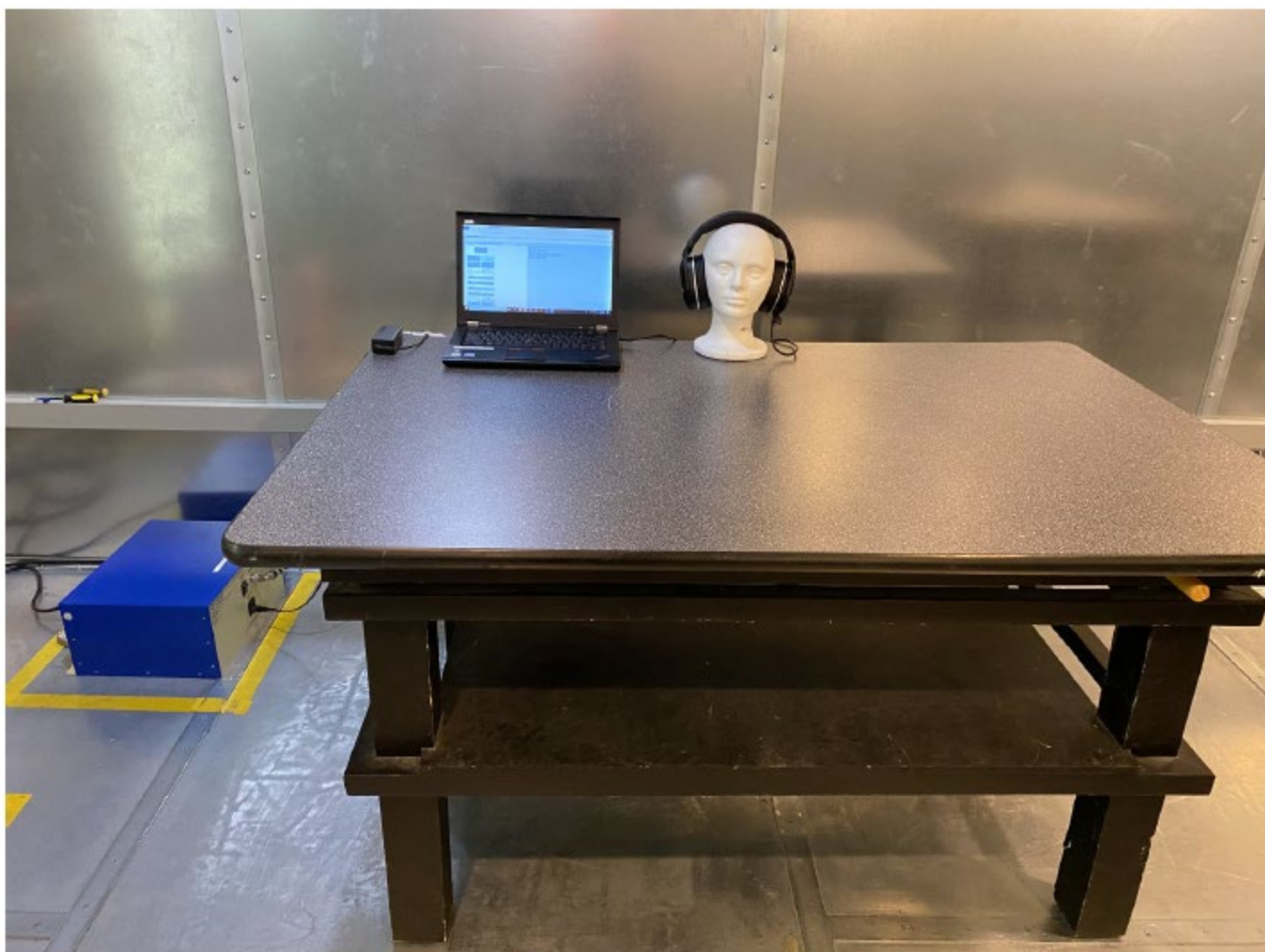
Figure 10: AC Conducted Emission Test Setup (Front View)
