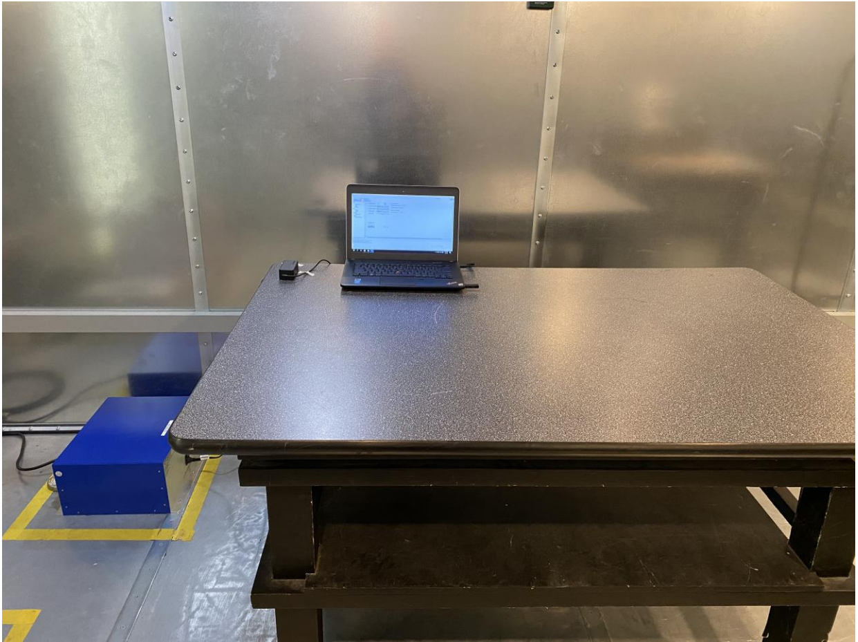
Figure 10: AC Conducted Emission Test Setup (Front)
