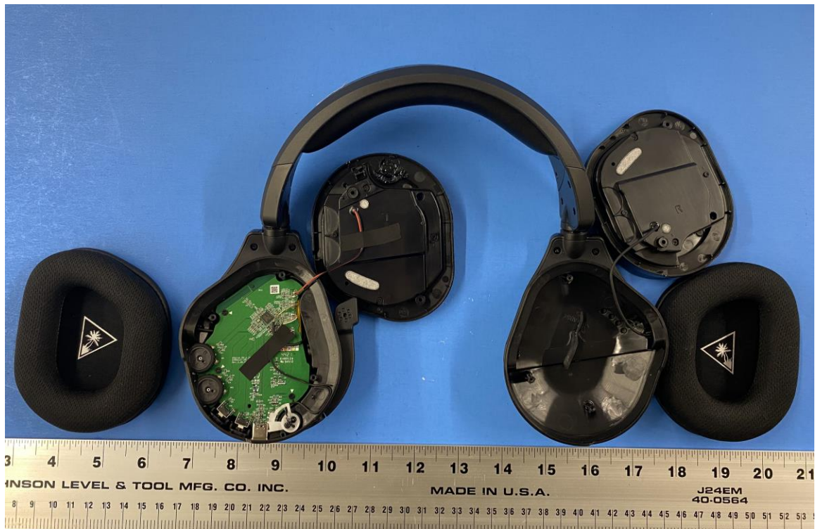
Figure 1: Internal Photo of Stealth600X-USB-RX - Remove Speakers
