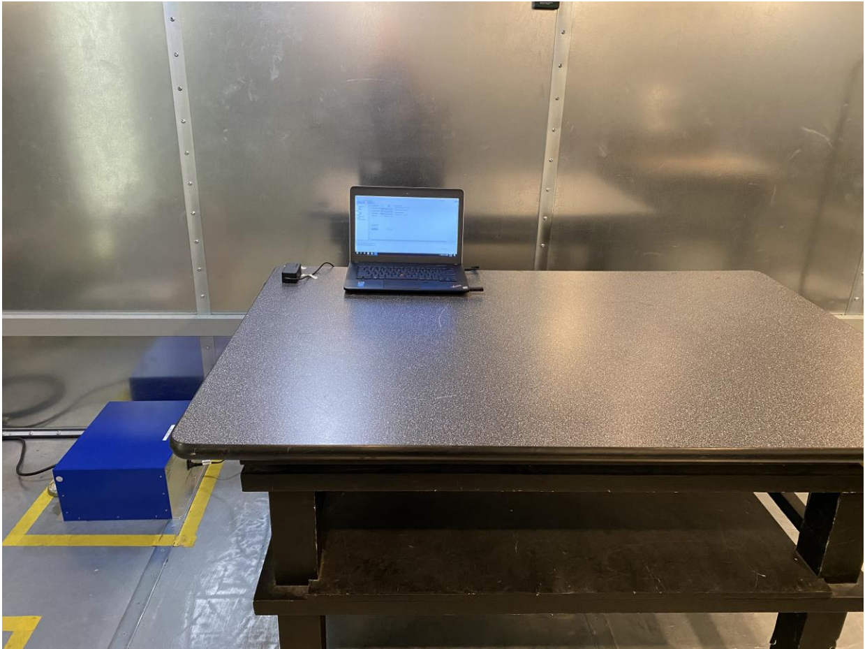
Figure 10: AC Conducted Emission Test Setup (Front)
