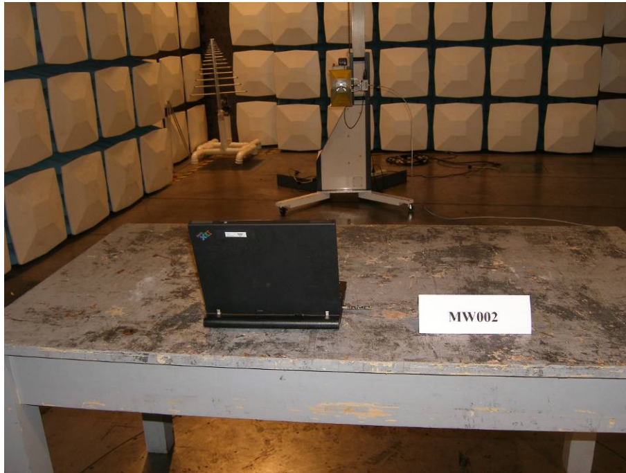
Photograph 2: Set-up for Radiation Measurement above 1GHz
