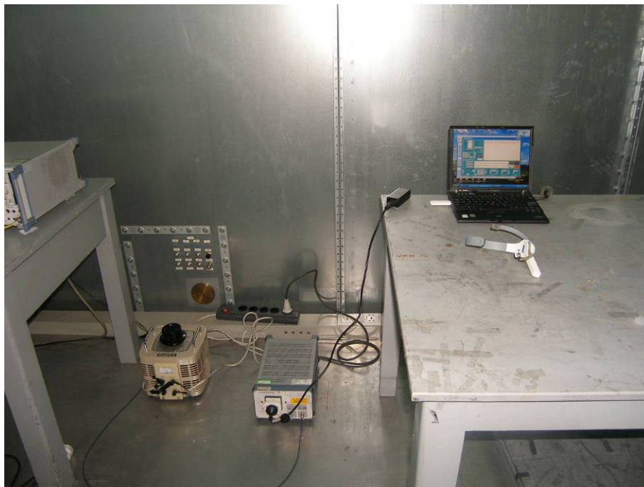
Photograph 3: Set-up for AC mains conducted emission
