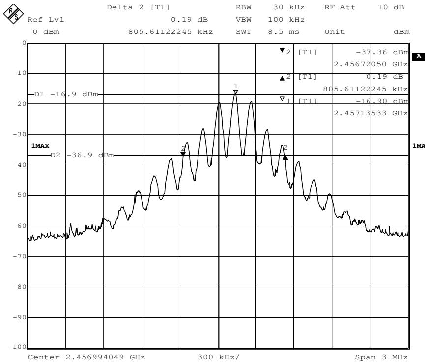
**3. Test R6 transceiver in the highest frequency 2.476.989166 GHz**
