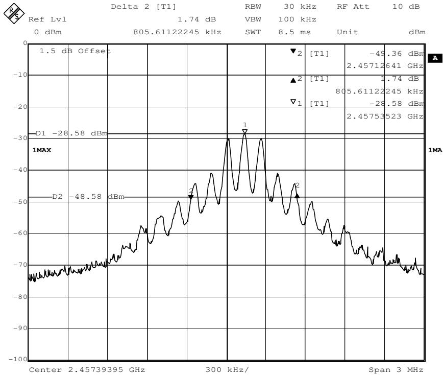
**3. Test R4 transmitter in the highest frequency 2477.389069 GHz**
