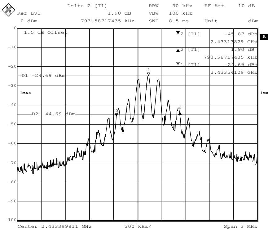
**2. Test R4 transmitter in the middle frequency 2.457.393951 GHz**
