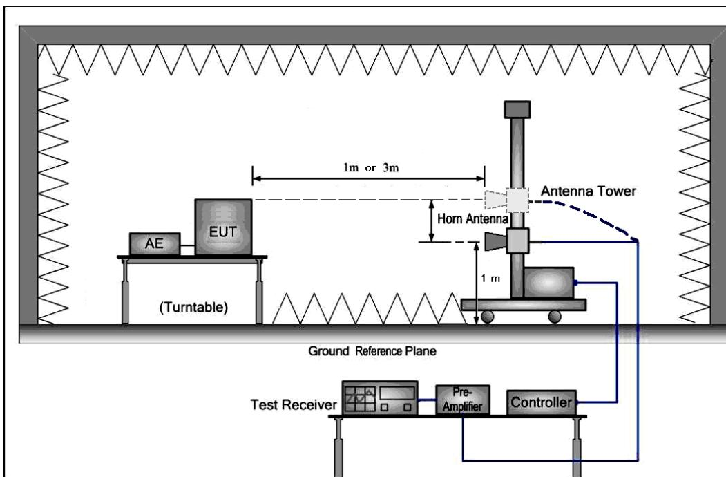
The field strength is calculated by adding the Antenna Factor, Cable Loss & Per-amplifier. The basic equation with a sample calculation is as follows:
