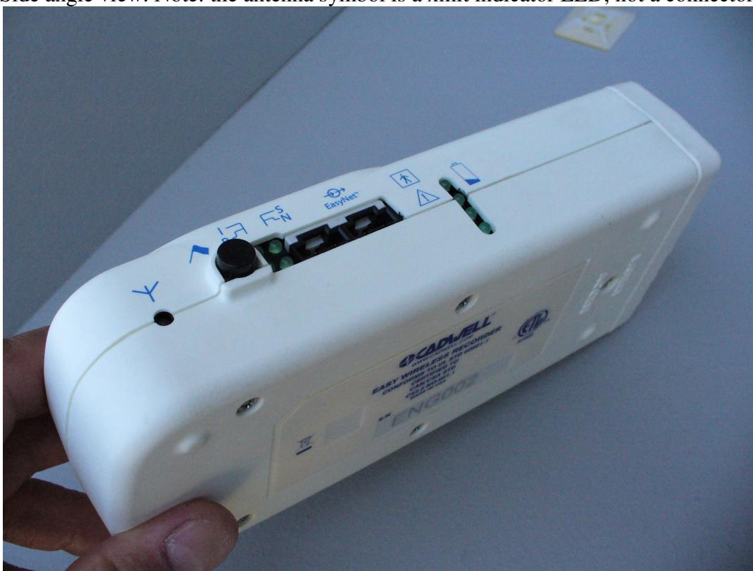
Battery pack and wired Ethernet quick disconnect adapter removed
