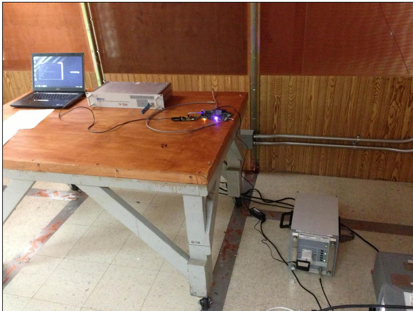
Photograph 19. Conducted Emissions, §15.315, Test Setup
