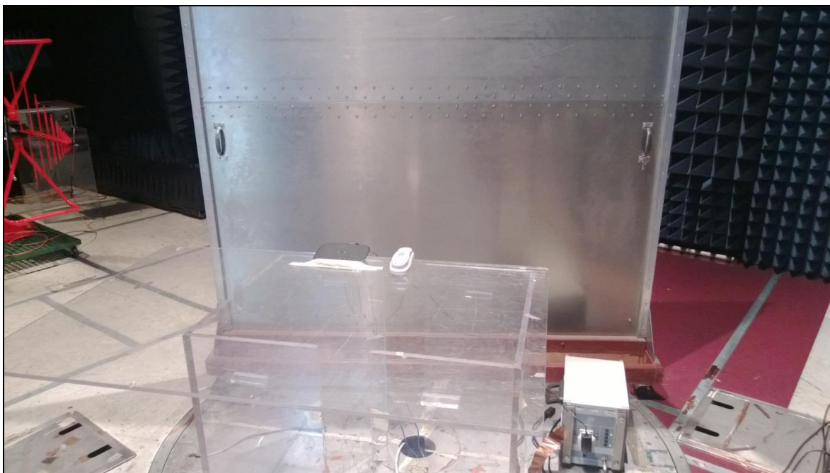
Photograph 10. Conducted Emissions, Test Setup, Telo
