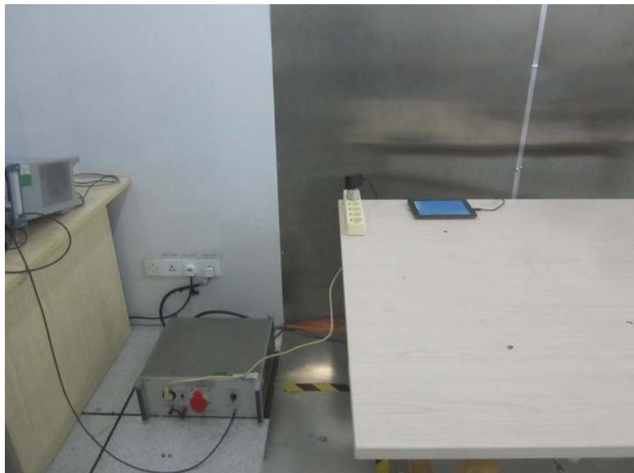
**Radiation Emission Test Setup (Below 30MHz)**
