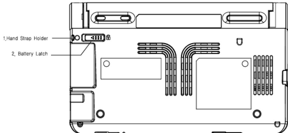
**Battery latch** The latch used to remove or install the battery.
