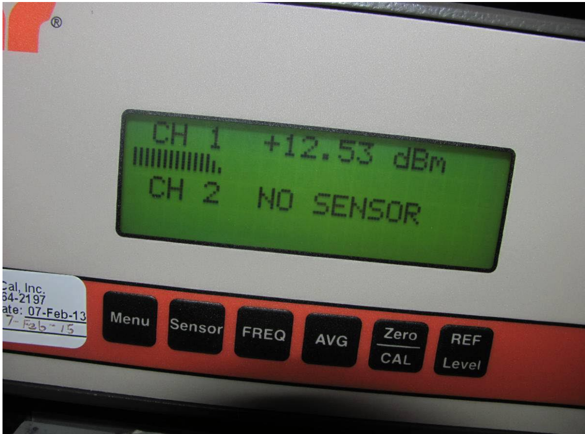
Figure 3: Maximum power of Lo, Mid, and Channel 25 using -11 dBm (actual power) setting in SW
