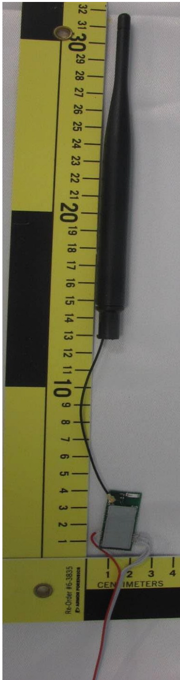
Illustration 3: EUT with external whip antenna
