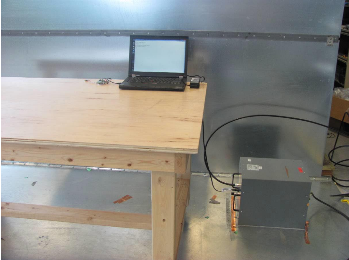
Illustration 10: Power line conducted emission setup – photo 1
