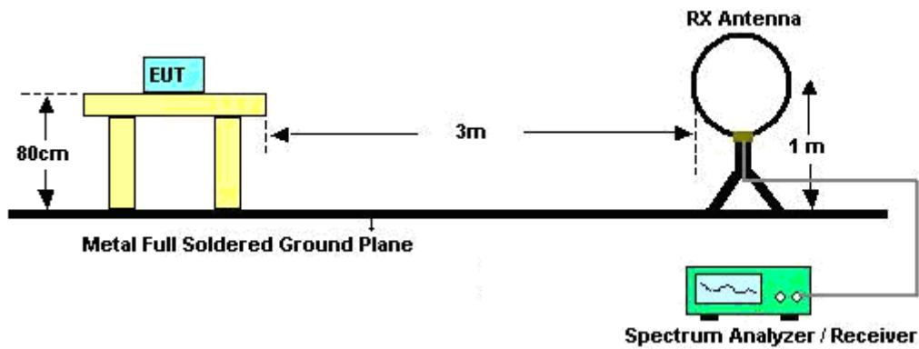
For radiated emissions from 30MHz to 1GHz
