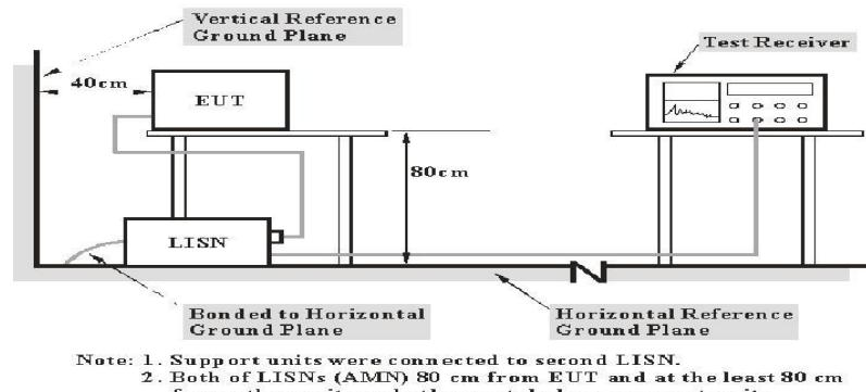
The setup of EUT is according with per ANSI C63.10-2013 measurement procedure. The specification used was with the FCC Part 15.207 limits
