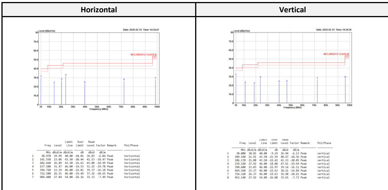
*Level = Reading Level + Correct Factor*
