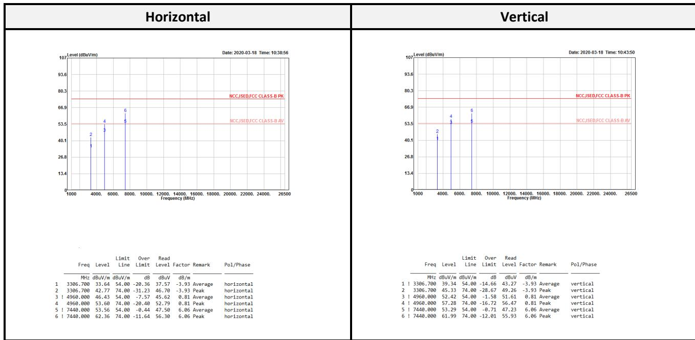
*Level = Reading Level + Correct Factor*
