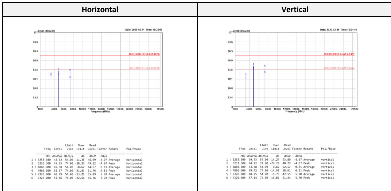
*Level = Reading Level + Correct Factor*
