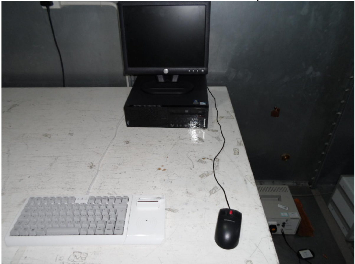
Measurement of Conducted Emission Test Set Up
