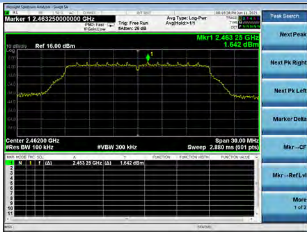
802.11n-20 MHz HIGH CHANNEL, Carrier level
