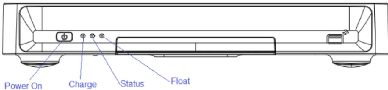
The MTRAY-F1 has different LEDs to indicate the reader status.
