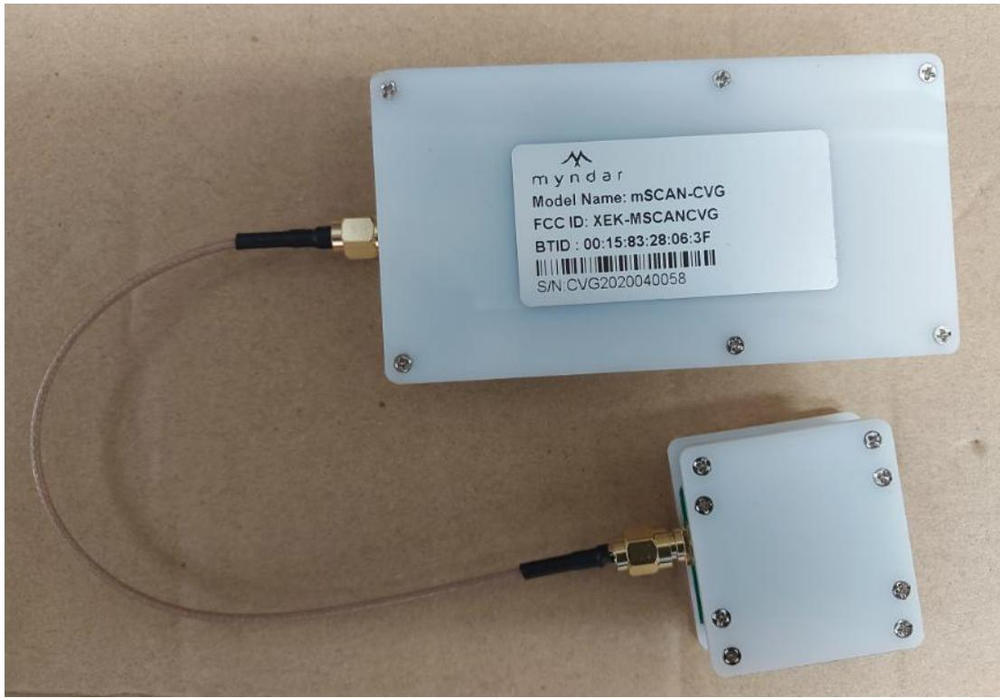
MSCAN-CVG is an UHF EPC C1G2 portable RFID reader. It is designed for close proximity reading. It is a compact RFID reader and OS independent with Bluetooth connectivity to any mobile devices. It serves as a handy checkpoint at different stages throughout the value chain, such as logistics operations, inventory management and POS system etc.
