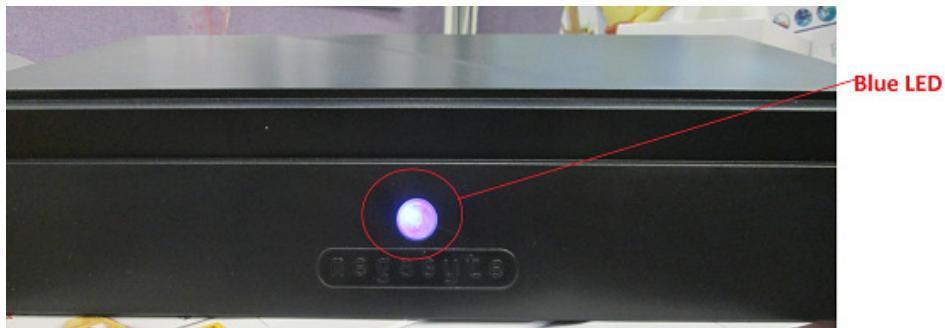
The Logistic Tray L2-U has different LEDs to indicate the reader status.
