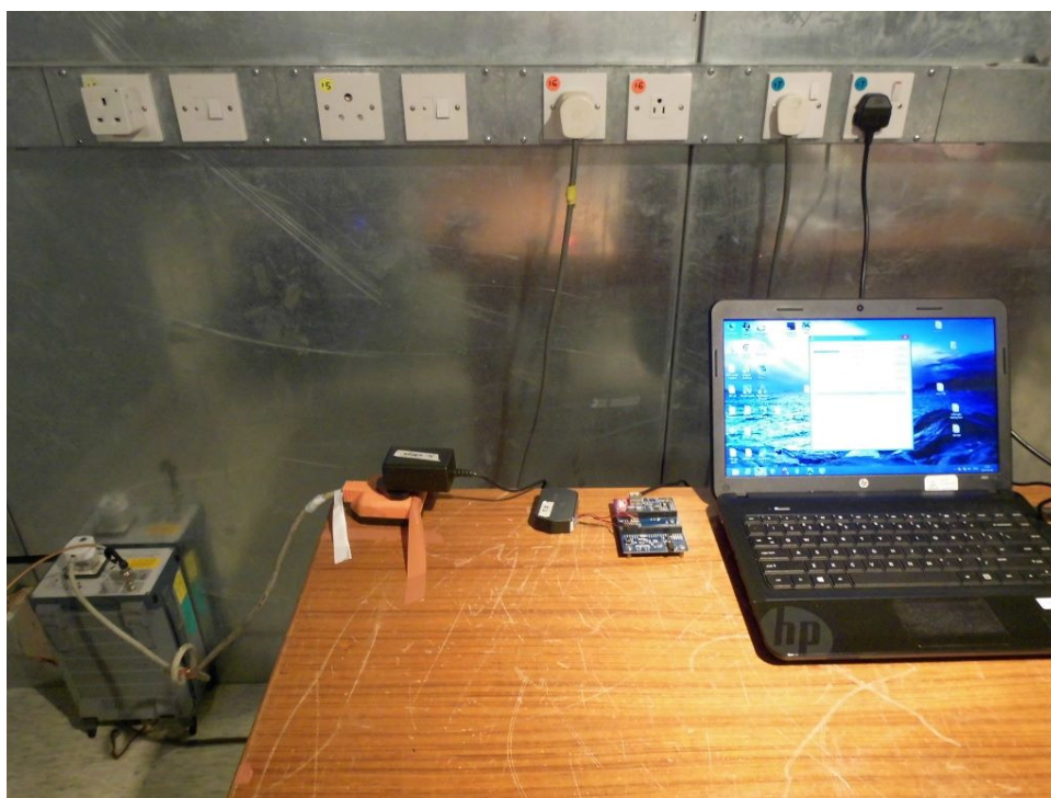
Set-up for AC Mains Conducted Emission
