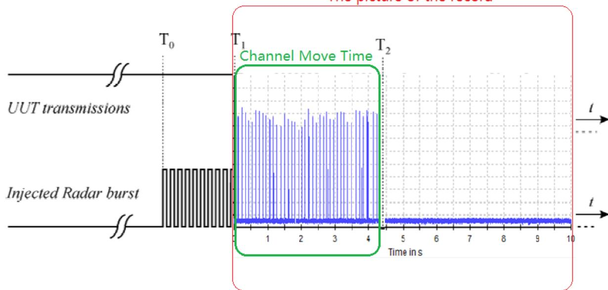
$T_0$  denotes DFS test signal start generated on the channel.
