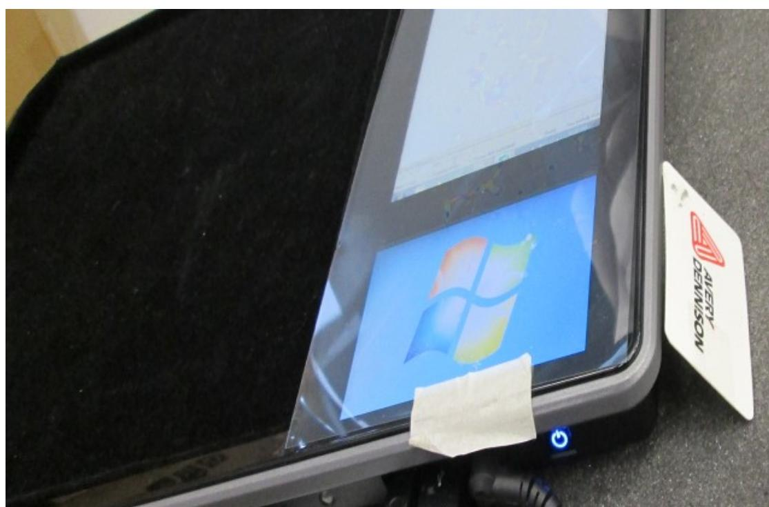
**X.** 39-T1 operates at UHF frequency band, ranging from 865MHz to 928MHz (ETSI 865-868 MHz, FCC 902-928 MHz, SRRC 920-925 MHz and NCC 922-928 MHz); the setting depends on countries' regulations.
