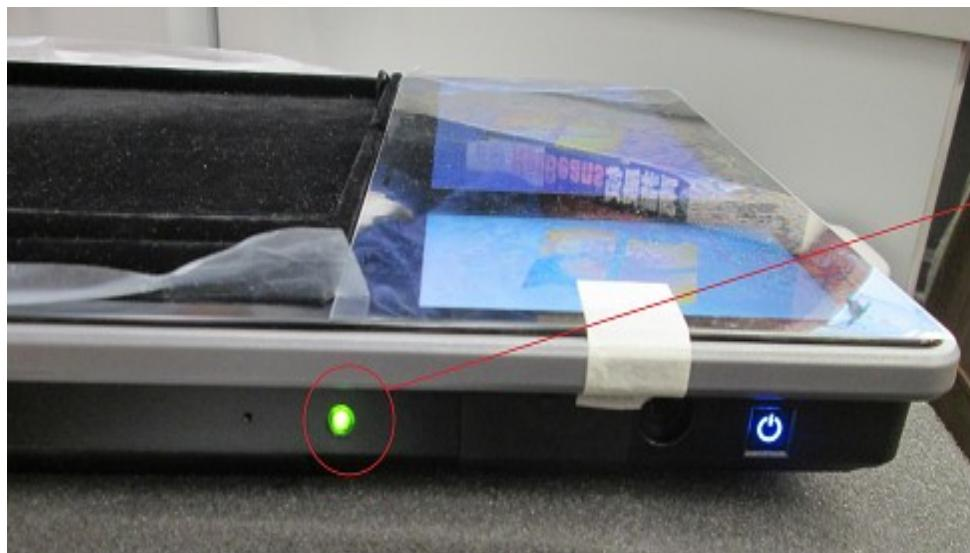
The 39-T1 has different LEDs to indicate the reader status.
