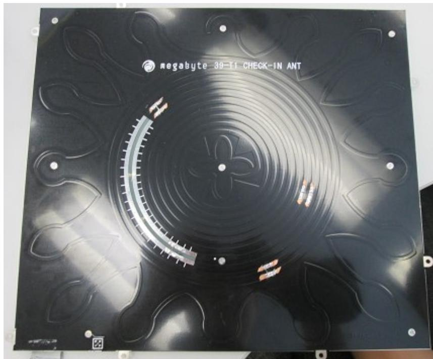
**Checkout antenna: antenna gain = 0dBi**
