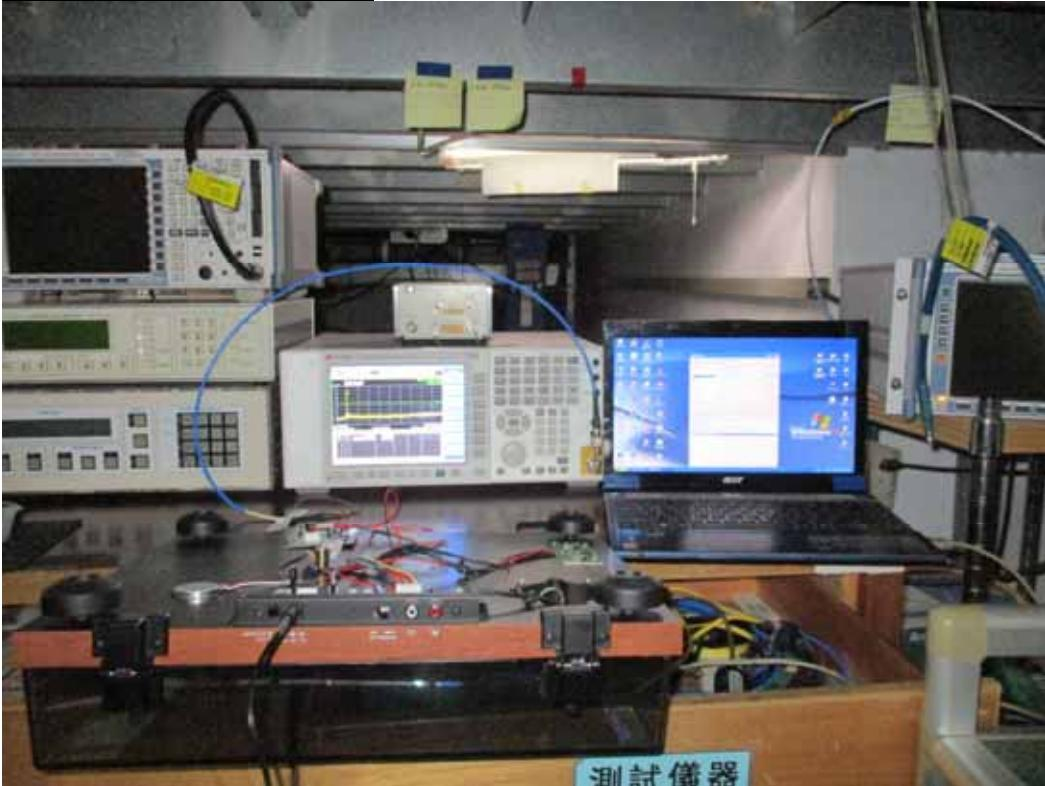
**CONDUCTED EMISSION MEASUREMENT SETUP**
