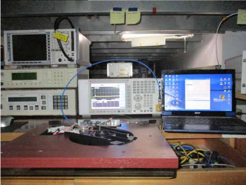
**CONDUCTED EMISSION MEASUREMENT SETUP**
