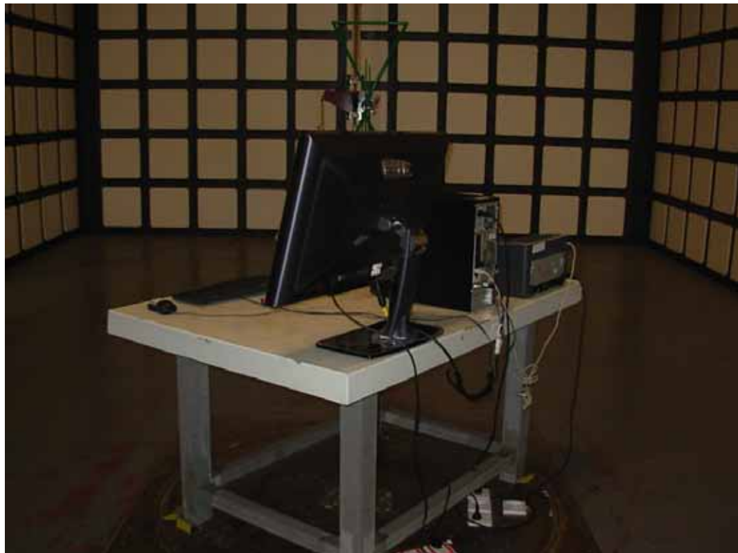
SETUP WITH MAXIMUM DETECTED EMISSION AT VERTICAL POLARIZATION (DP TO DVI 1680*1050@60Hz)
