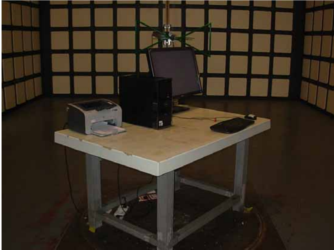
SETUP WITH MAXIMUM DETECTED EMISSION AT HORIZONTAL POLARIZATION (DP TO DVI 1680*1050@60Hz)
