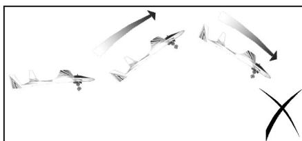
b) If the plane raises its nose very quickly, it may fly near stalling speed and fall down. You should pull the left lever down (throttle down) to let it fly in horizontally.
