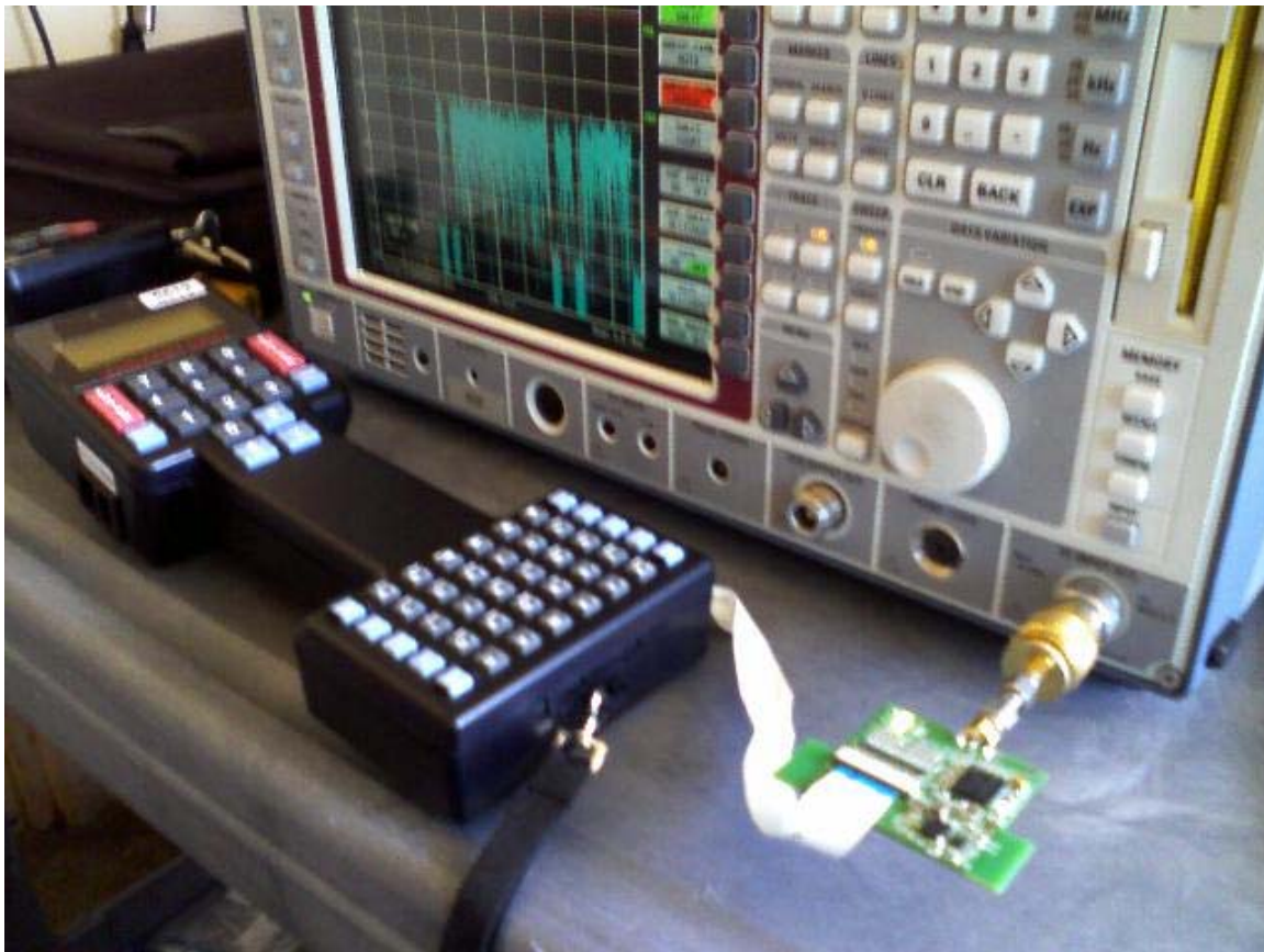
Antenna replaced by sma connector for conducted tests.
